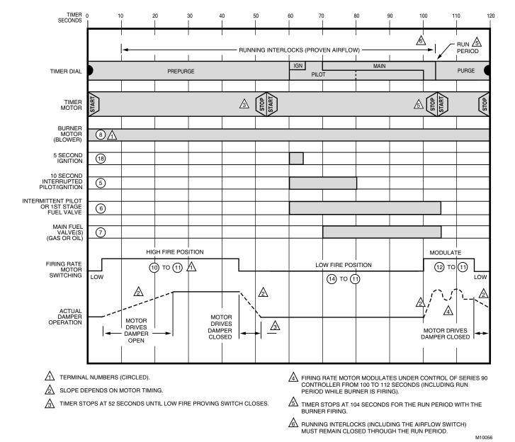
Fig. 10. Timer sequence for R4140G1056 and R4140G1064 Programmers.
